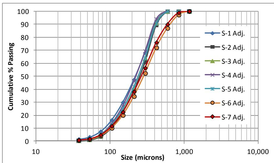
Figure 13-14: Particle Size Distributions for Pilot Plant Final Concentrate
