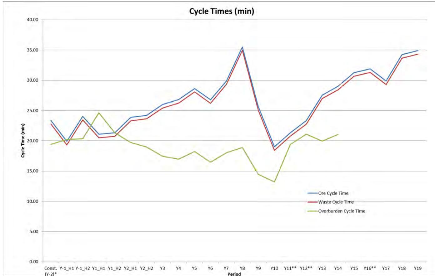
Figure 16-33: Cycle Time by Material Type
