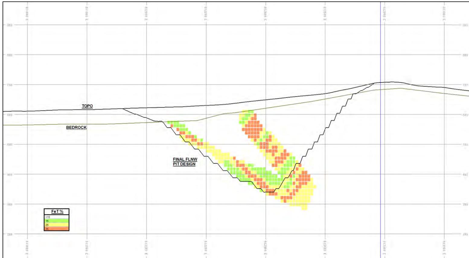
Figure 15-11: FLNW Pit Section View N 5 808 500 m
