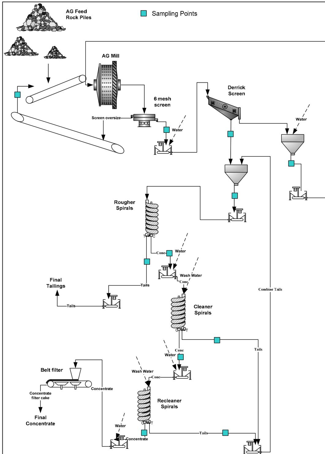
Figure 13-5: Schematic Pilot Plant Flowsheet (runs C-1 and S-1 to S-6)
