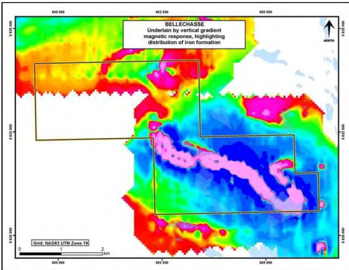
**Figure 7-11: Magnetic Vertical Derivative Geophysical Map of Bellechasse**
