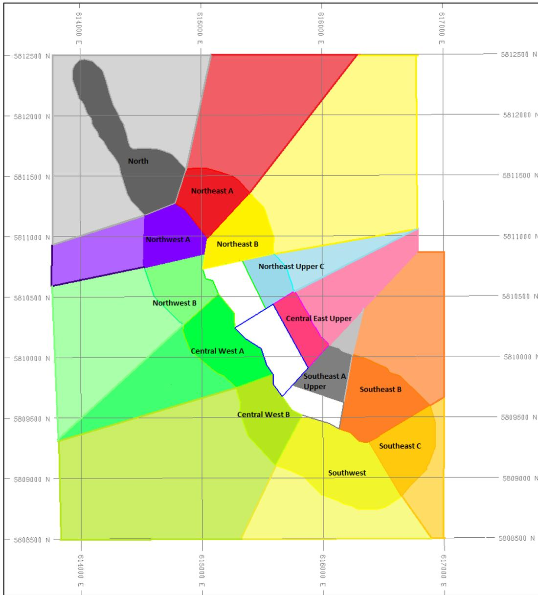
**Figure 15-7: Fire Lake North East Pit Slope Sectors**
