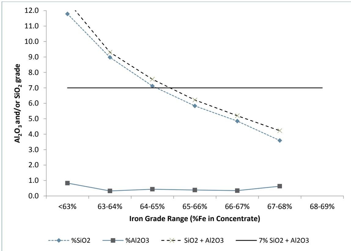
Figure 13-10: East Pit  $\text{SiO}_2 + \text{Al}_2\text{O}_3$  Levels vs. Fe Concentrate Grade (100% Passing 20 Mesh)
