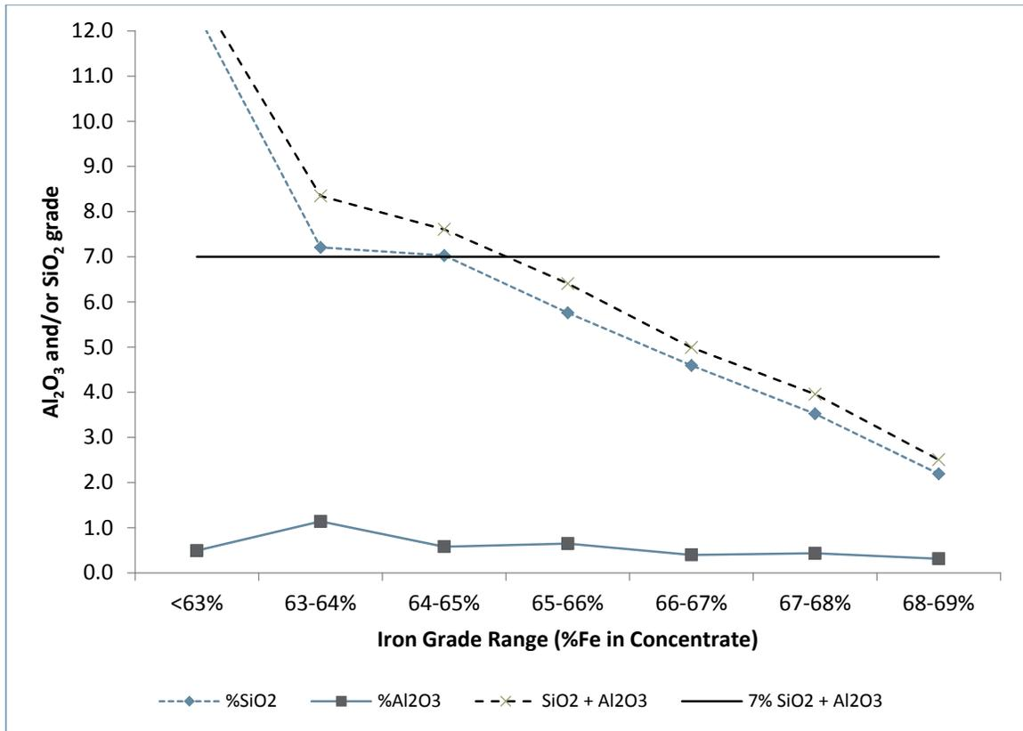
Figure 13-9: West Pit  $\text{SiO}_2 + \text{Al}_2\text{O}_3$  Levels vs. Fe Concentrate Grade (100% Passing 20 Mesh)
