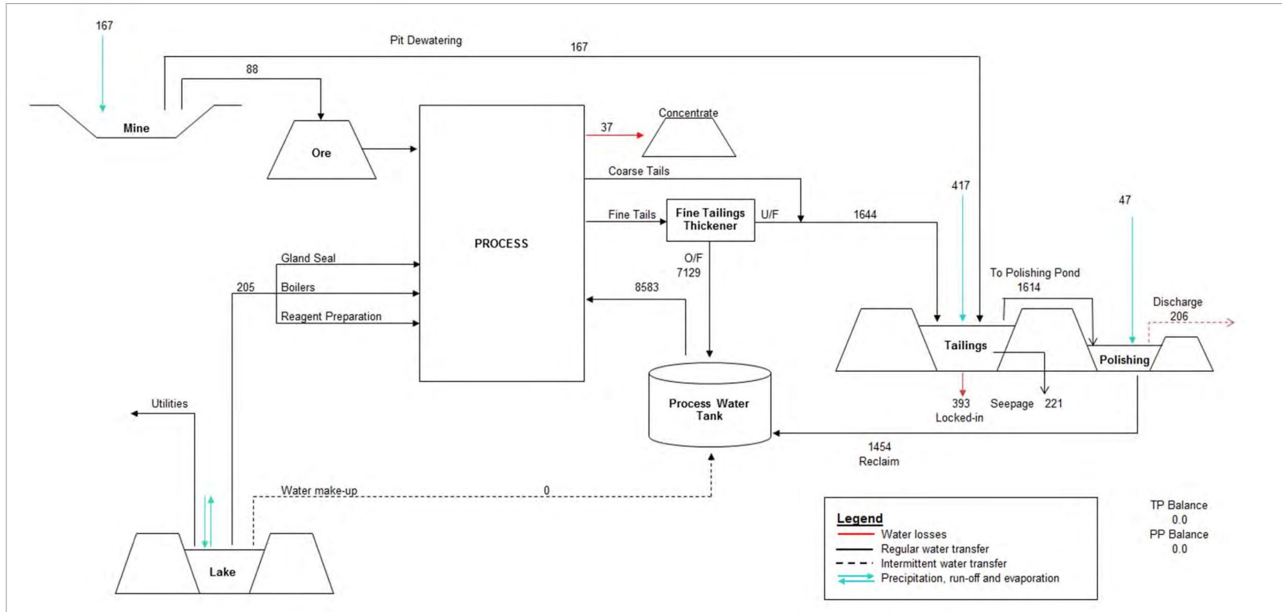
Figure 17-3: General Process Plant Water Balance
