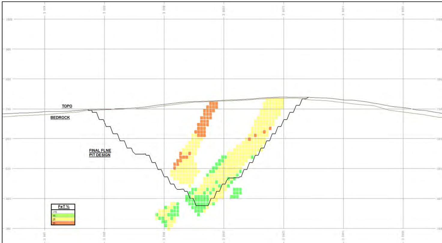
Figure 15-16: FLNE Pit Section View N 1500 m
