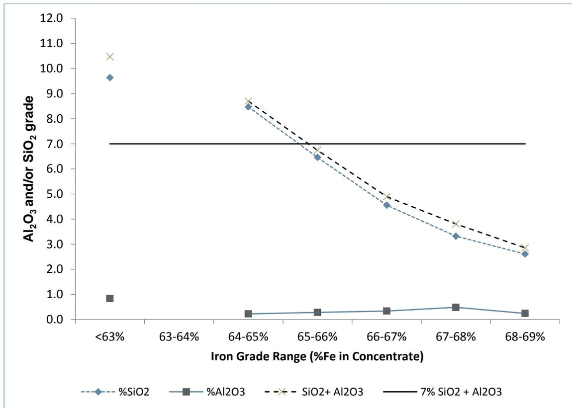
**Figure 13-11: East Pit SiO<sub>2</sub>+Al<sub>2</sub>O<sub>3</sub> Levels vs. Fe Concentrate Grade(100% passing 28 Mesh)**
