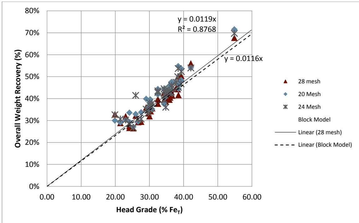
**Figure 13-8: East Pit Head Grade vs. Weight Recovery**
