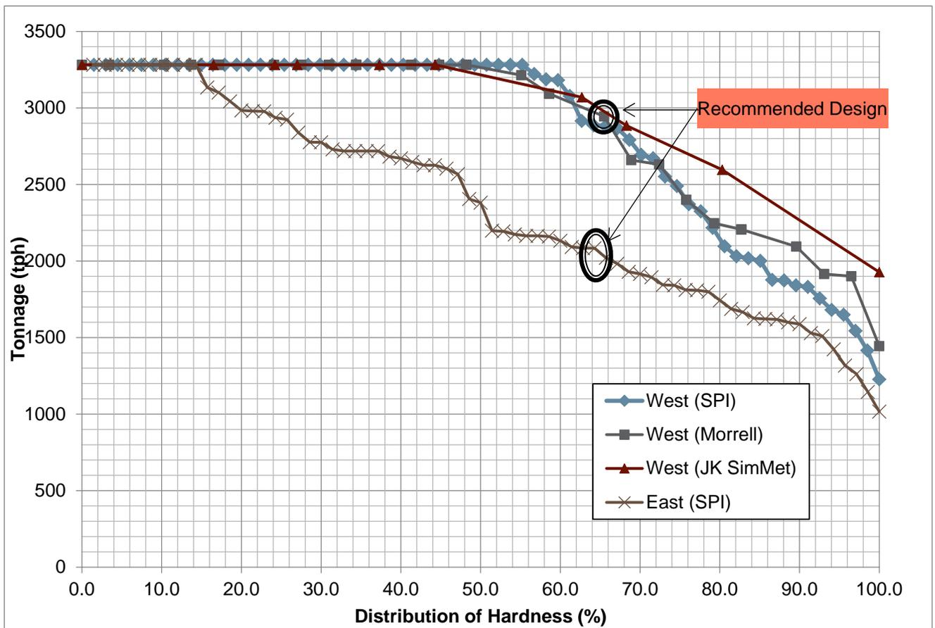
Figure 13-4: Throughput Analysis for West and East Pits
