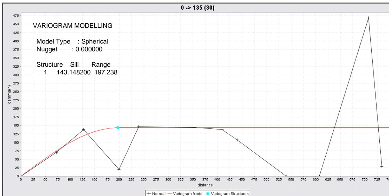
**Figure 14-17: Directional Semi-Variogram (Azimuth 135°)
