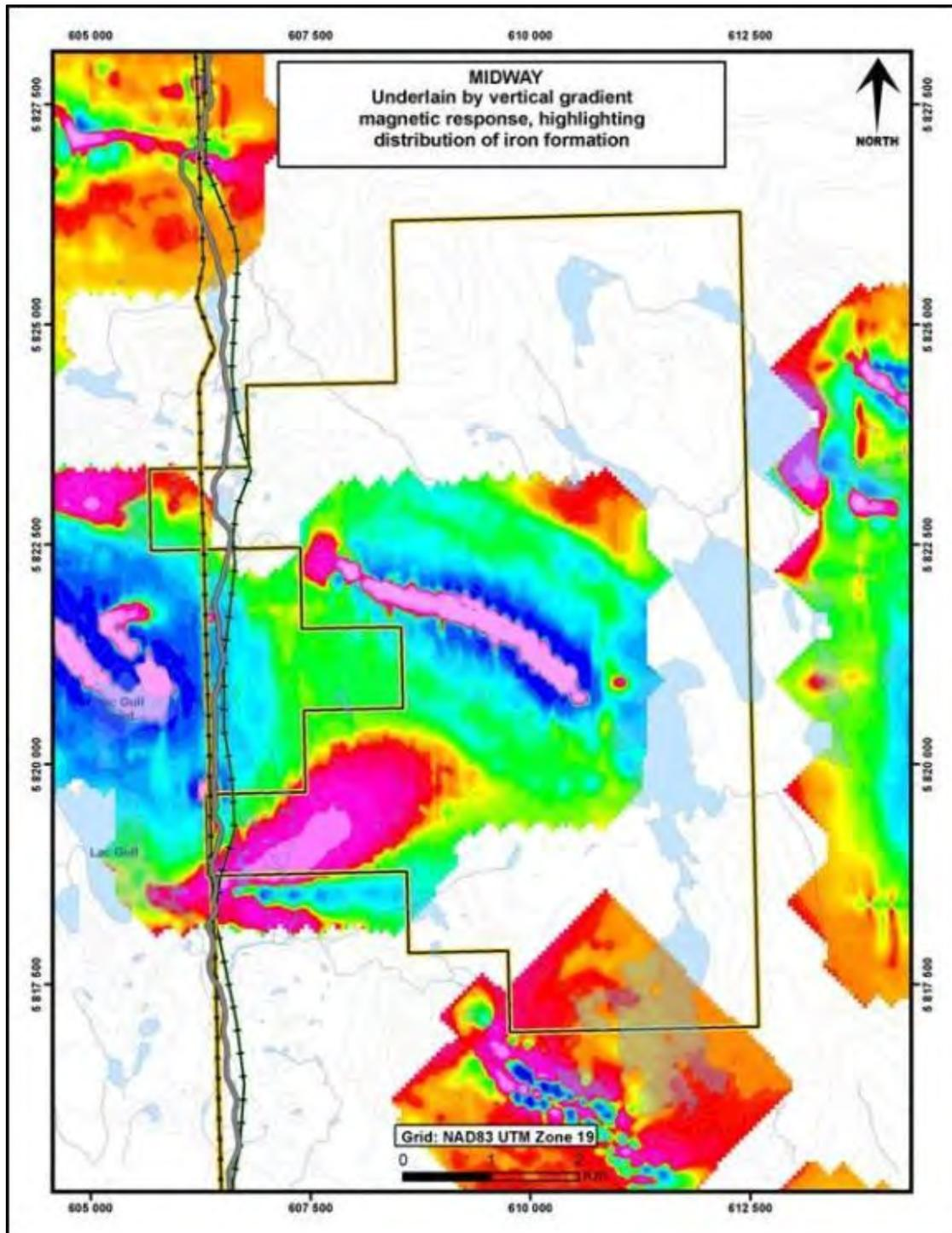
Figure 7-13: Magnetic Vertical Gradient Geophysical Map of Midway
