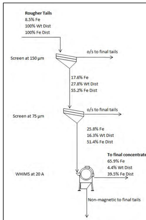
**Figure 13-15: Material Balance of Fine Iron Recovery Testwork**
