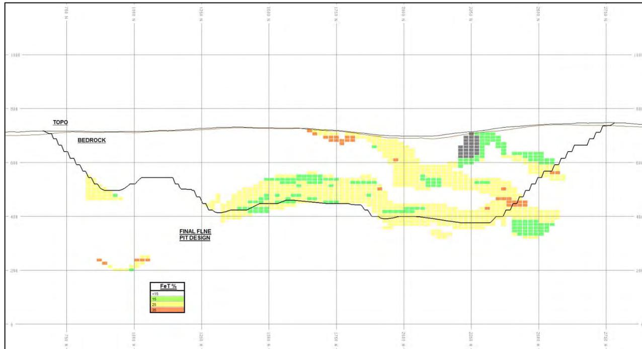
Figure 15-18: FLNE Pit Section View E 1000 m
