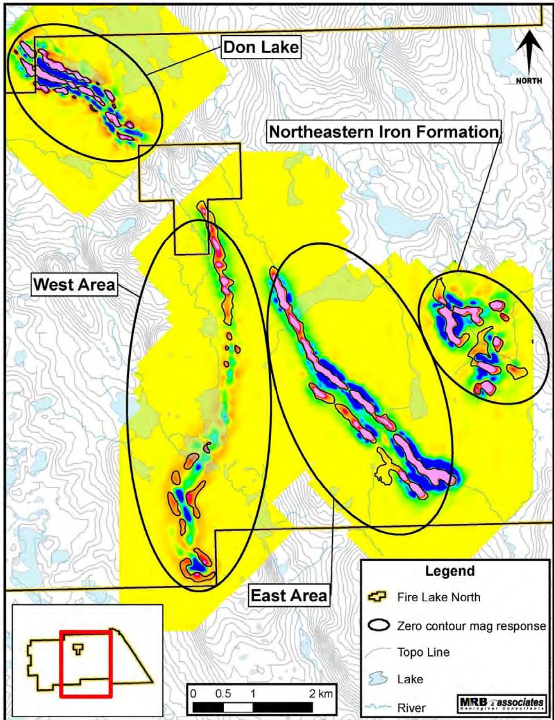
Figure 7-7: Magnetic Second Vertical Derivative Geophysical Map of Fire Lake North
