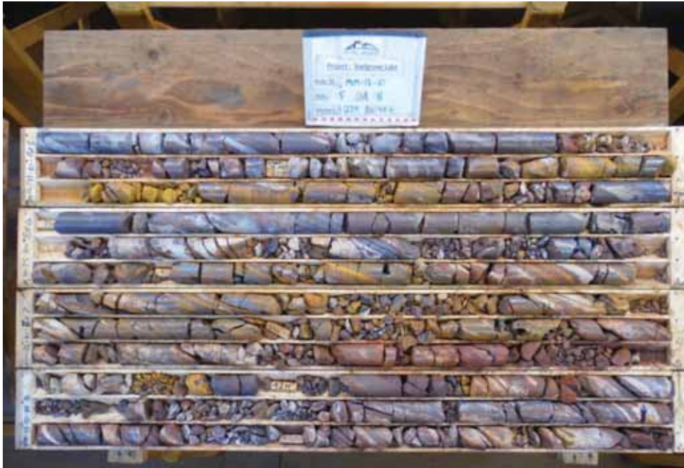
Figure 10-9: Photo of MM-13-10 - CLC North - Core recovered from 27.4-45.6m
