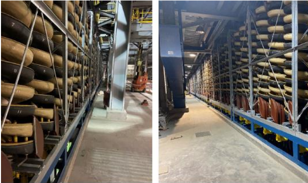
Concentrator – Spirals and launders installation
