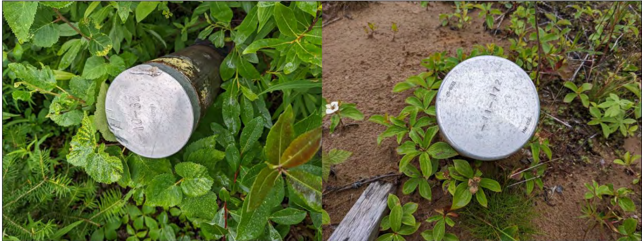
Figure 12-2: Example of Drillhole Collars (K-10-32 and K-11-172)
