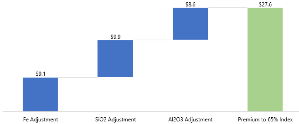
Figure 19-4: VIU premium to P65 Index estimate for chemical characteristics of the Kami Product
